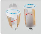
4 Attach C3 and C4 in turn to B7, and attach C5 and C6 in turn to B8.
