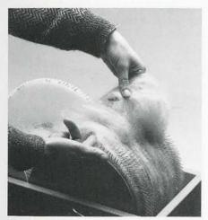
11 To remove the wool, insert a finger or knitting needle under the combed layer at the opening across the drum.
