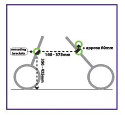
You cannot fit a bracket around two parallel telescopic tubes, as the tubes may slide alongside each other or split apart when folding pushchair (e.g. Bebeconfort Loola).
